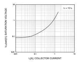
Figure 2. Collector-Emitter Saturation Voltage
