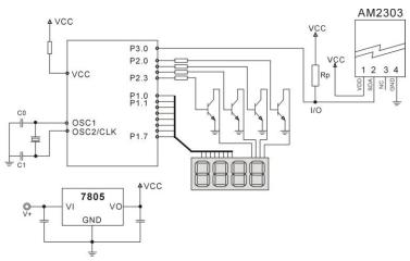
Pic4: AM2303 Typical circuits for single bus
