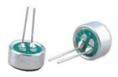
Electret microphone is a type of condenser microphone. Operating voltage: 3Vdc Operating voltage range:1.5V-10Vdc Sensitivity:-48dB~+66dB Operating Current:500uA(MAX) Diameter size:9.7mm x 4.5mm (contains 2 pins) Directivity:Omnidirectional condenser microphone
