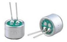
Electret microphone is a type of condenser microphone. Operating voltage: 3Vdc Operating voltage range:1.5V-10Vdc Sensitivity:-48dB~+66dB Operating Current:500uA(MAX) Diameter size:9.7mm x 6.7mm (contains 2 pins) Directivity:Omnidirectional condenser microphone
