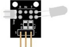
Pulse monitor works as follows: The LED is the light side of the finger, and photo transistor on the other side of the finger, photo transistor used to obtain the flux emitted,
