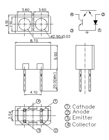
Note: Tolerances unless dimensions ±0.25mm
