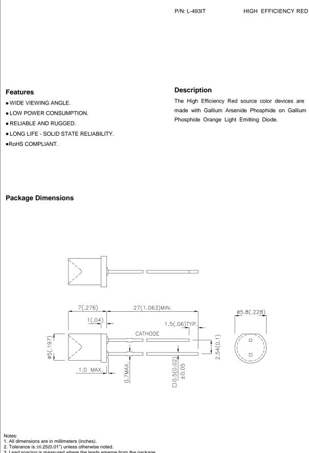
3. Lead spacing is measured where the leads emerge from the package.
