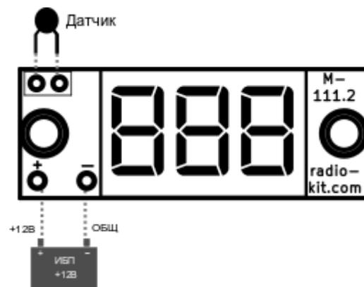
Attention: The sensor sealed to the board may show a few degrees more due to the heating of the module itself. In order to avoid unwanted heating of the sensor, it is necessary to connect to the module with the help of two wires.
