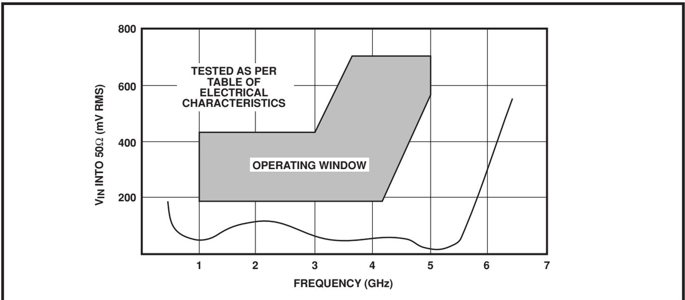
Figure3 Typical input sensitivity (sinewave drive)
