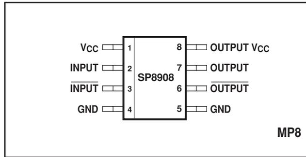
Figure 2 - Pin connections - top view
