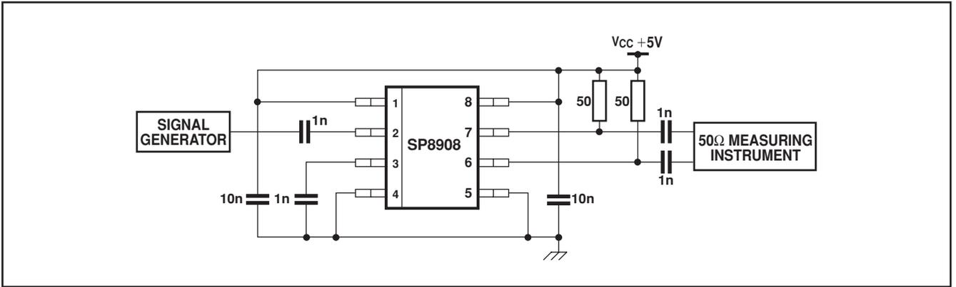
Figure 4 - Typical application and test circuit
