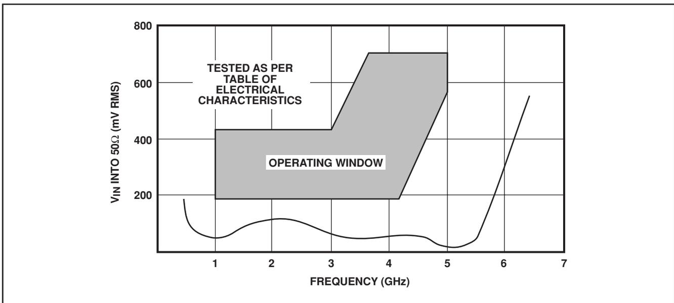
Figure 3 - Typical input sensitivity (sinewave drive)
