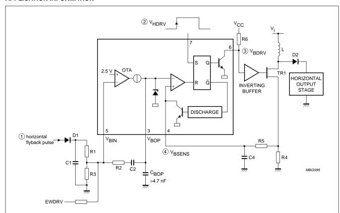
For f < 50 kHz and C2 < 47 nF calculation formulas and behaviour of the OTA are the same as for an OP. An exception is the limited output current at BOP (pin 3). See Chapter "Characteristics", Row Head "B+ control section (see Figs 12 and 13)".
