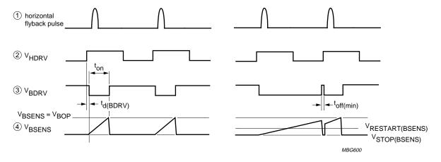
b. Waveforms for normal operation.
