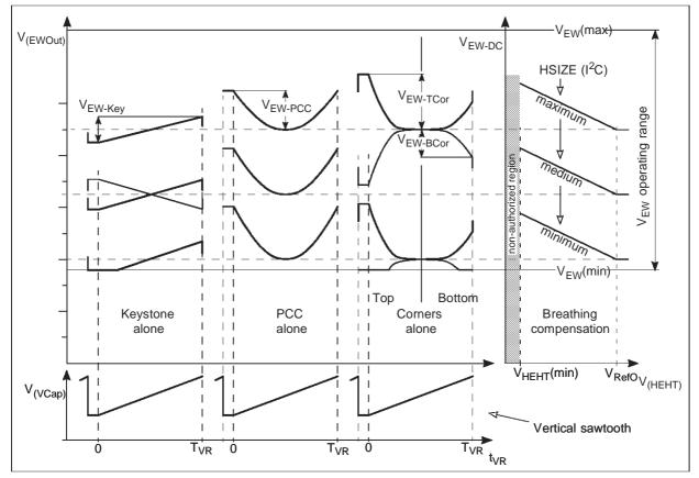
Figure 13. EWOut output waveforms
