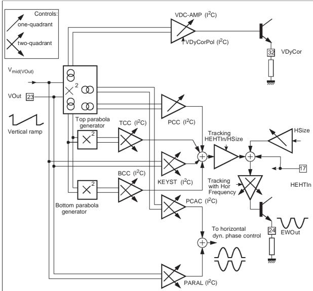
Figure 12. Geometric corrections' schematic diagram
