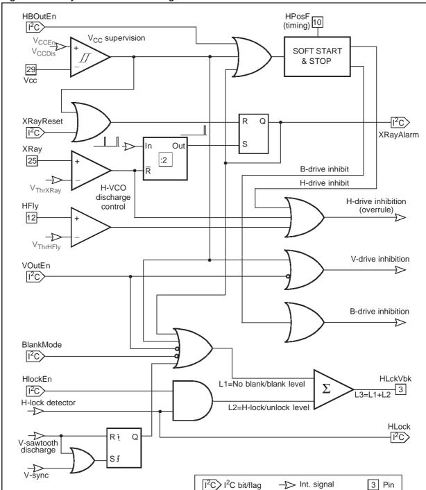
Figure 15. Safety functions - block diagram
