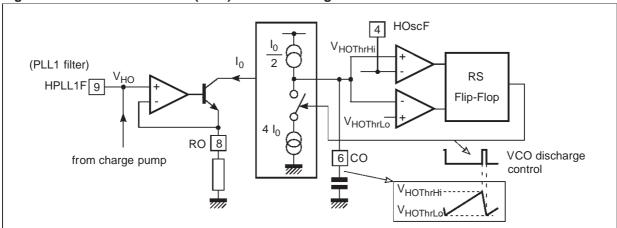
Figure 6. Horizontal oscillator (VCO) schematic diagram
